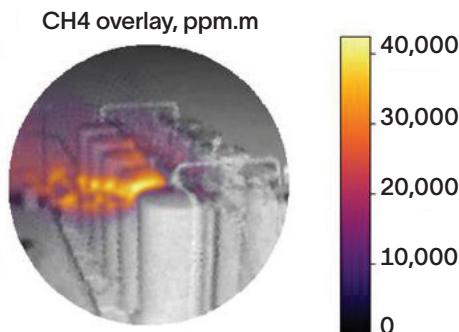
The methane lidar camera provides an image of a methane plume overlaid on a picture of the facility, clearly identifying the emission source.
