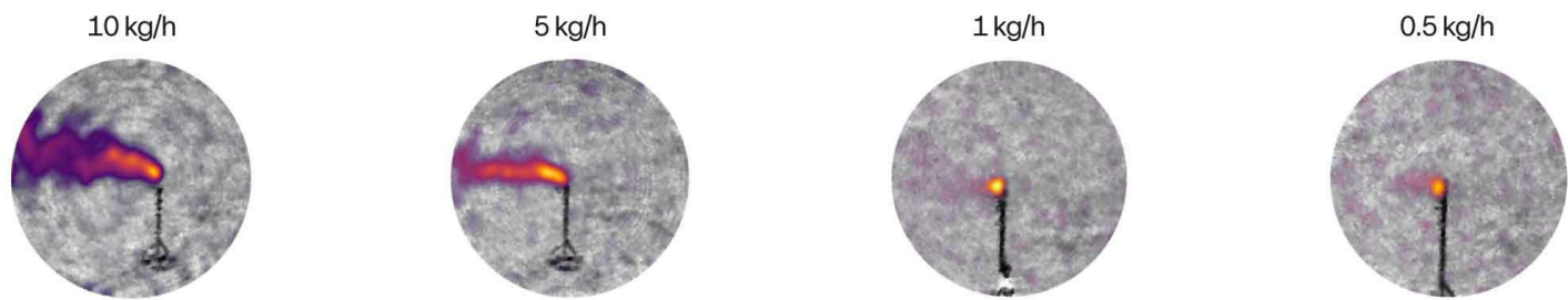
Larger emissions create larger methane plumes—enabling the methane lidar camera to quantify the emission rate.
