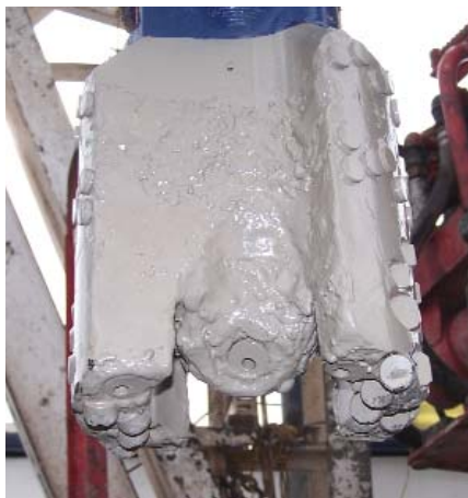
Figure 2. In field tests the PID system drilled hard rock at three to six times faster than conventional methods.
