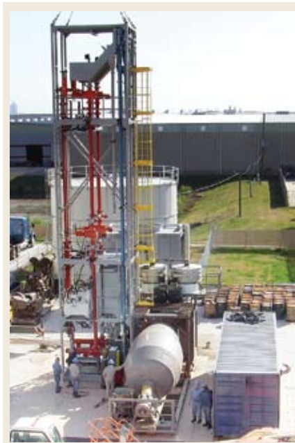
Fig. 7. The new injection method moves particles into the standpipe mechanically with a extruder-screw system.
