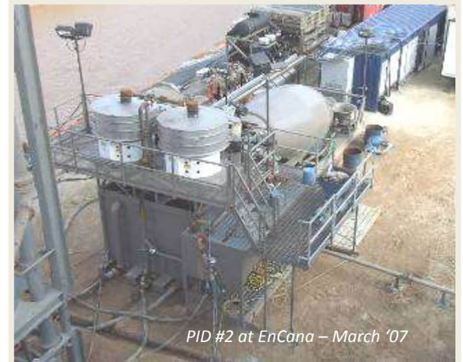
Components of the Hydraulic "frac pump" Injector System
