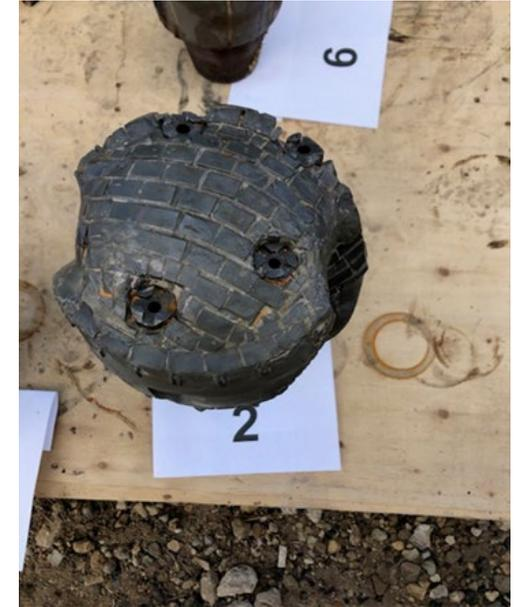
Used Particle Drilling PDT 44
